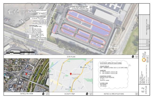
**Delivery Point:** Point of Delivery at new SCE 12kV switch located on riser pole near existing utility pole #1011362E
